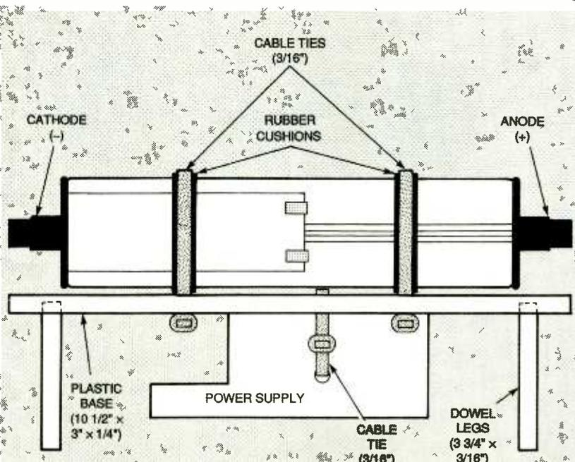
FIG. 4— ANOTHER VIEW OF HOW THE LASER TUBE is fastened to its platform. For safety reasons, it is best to place the laser tube inside a plastic or metal housing.
