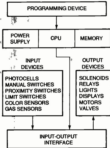
**FIG. 3—TYPICAL SYSTEM COMPONENTS** that are used in PLC industrial control systems.
