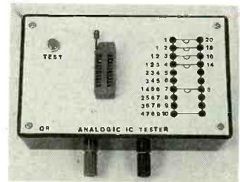
This inexpensive and easy-to-build tool lets you verify the operation of both analog and digital integrated circuits.
