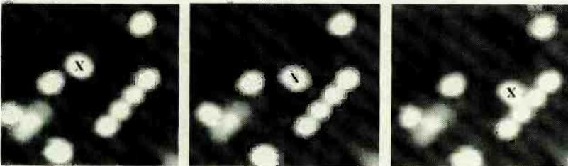
SANDIA ATOM TRACKER LOCKS ON TO A SILICON DIMER (marked with an "X") as it moves along a crystalline row of in-place silicon atoms.
