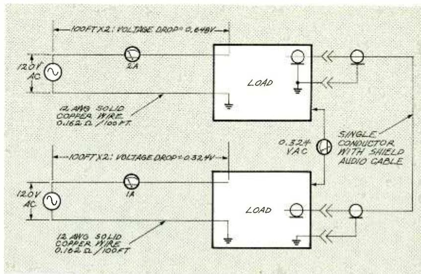
FIG. 2—VOLTAGE DIFFERENCE between two loads caused by different line voltage drops.
