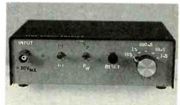
Convert your multimeter to a more useful tool by adding time-period measurement capability with this project.
