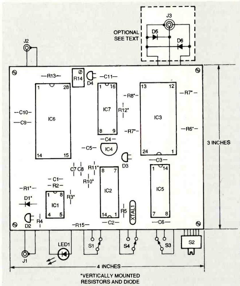
FIG. 2—PARTS PLACEMENT DIAGRAM. Panel-mounted components are shown schematically outside of the circuit board outline.
