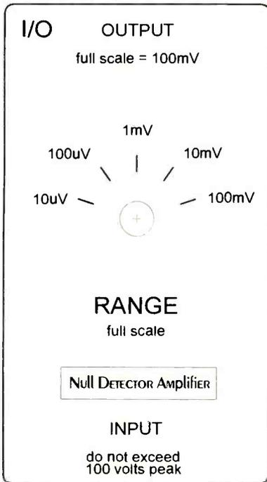
FIG. 4—FRONT PANEL suggested layout.
