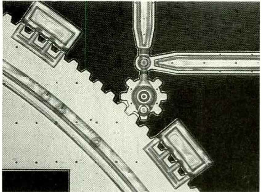
A MICROGEAR SMALLER THAN THE DIAMETER OF A HUMAN HAIR drives a gear 30 times larger than itself. Rectangular brackets stop the large gear, which acts as an optical shutter when light passes through the rectangular opening, from warping.
