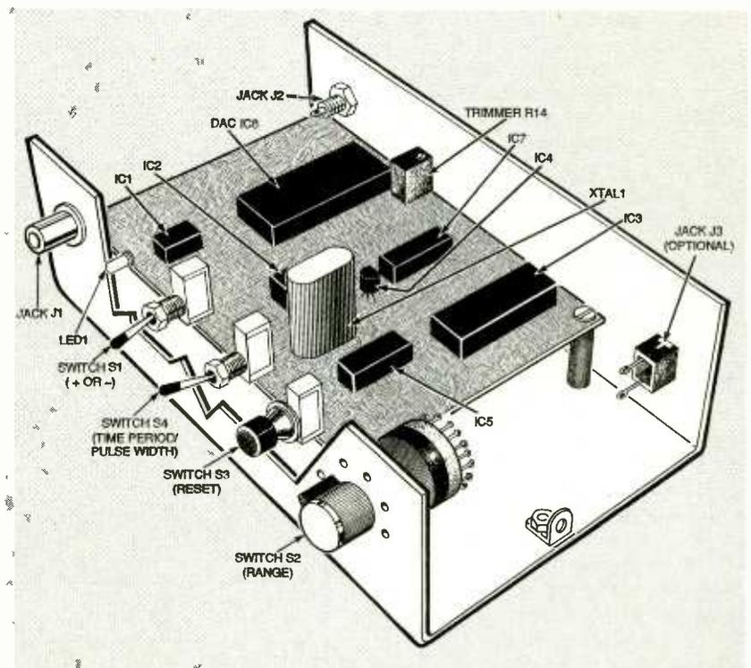
FIG. 4—ASSEMBLY DIAGRAM showing the location of principal components.
