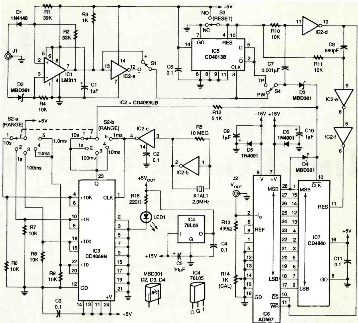
FIG. 1—SCHEMATIC FOR THE TIME PERIOD ADAPTER. Panel-mounted components are located on the front and back walls of the project case.
