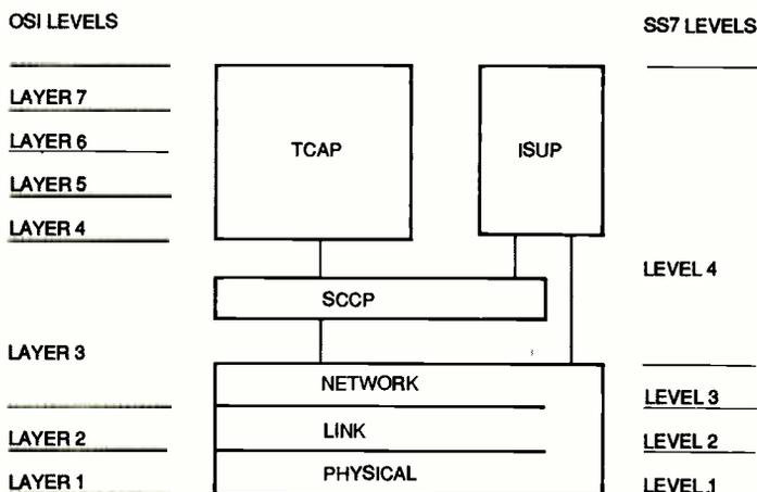
FIG. 3—OPEN SYSTEMS INTERCONNECTION (OSI) and Signaling System 7 (SS7) protocol models.
