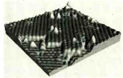
SCANNING TUNNELING MICROSCOPE VIEW of atoms in a silicon lattice with bumps on the surface showing deposited atoms.
