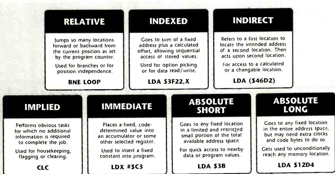
**FIG. 1—** THE KEY SECRETS to using and understanding microcontrollers and microprocessors lie in understanding and properly selecting addressing modes. Here are the seven most common addressing modes in use today.
