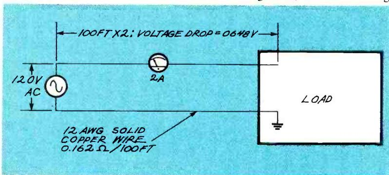
FIG. 1—POWER LINE voltage drop across a line, 100-feet long.
