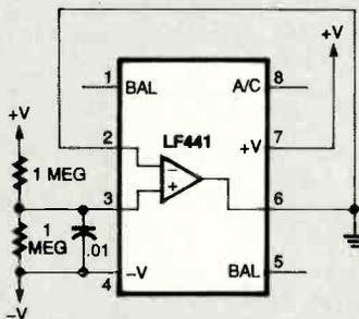
The circuit shown here should work fine. You must use a low-power op-amp, of which there are many to choose from. The National LF441 is a good, inexpensive choice (don't confuse it with the 411). Pin 6 is the virtual ground "output". This circuit will work correctly down to a battery voltage of about six volts. The current consumption is about 160 microamperes.
