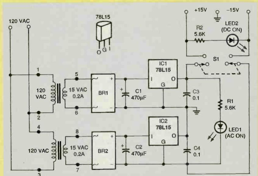
**SCHEMATIC FOR OPTIONAL  $\pm 15$ -VOLT dual power supply**
