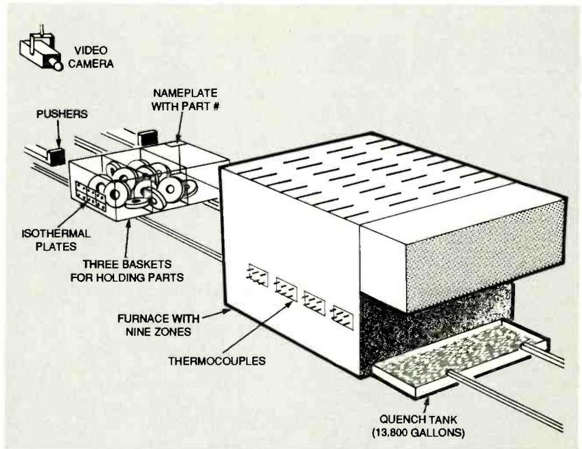
FIG. 8—THERMOCOUPLES MONITORING FURNACE TEMPERATURE. This is typical of how sensors are used to monitor industrial systems run by PLCs.
