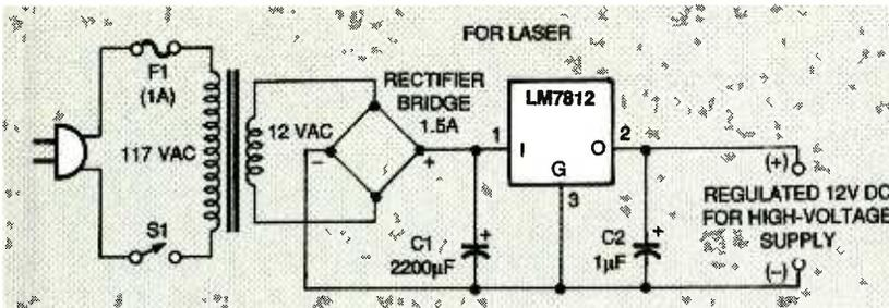
**FIG. 5—** REGULATED POWER SUPPLY DELIVERS 12 volts DC to drive the laser's high-voltage supply.
