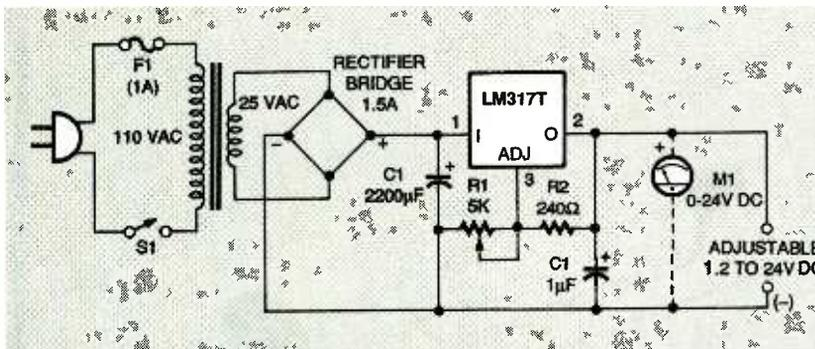
**FIG. 6—** A MORE ELABORATE VARIABLE POWER SUPPLY is shown here. The meter, which can be an analog or a digital type, is optional.
