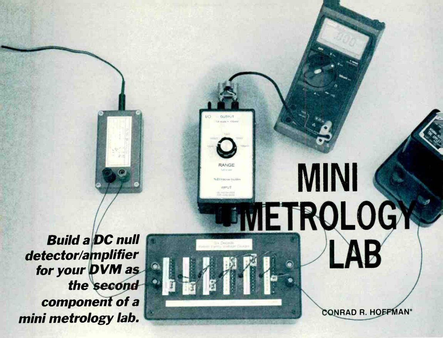
**Build a DC null detector/amplifier for your DVM as the second component of a mini metrology lab.**
