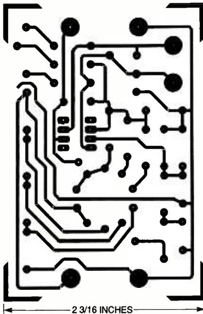
wiring errors, and will result in the most stable and reliable null detector. A circuit-board layout is provided here. Figure 3 is its parts-placement diagram.
