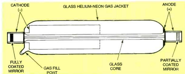
**FIG. 2— BASIC DIAGRAM OF AN He-Ne laser tube.** Some tubes have metal ends instead of the solid glass envelope. The glass fill port is used during manufacturing to charge the tube.
