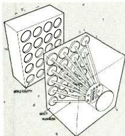
FIG. 10—PLASTIC INJECTION MOLDING SYSTEM. Thermocouples are installed in the injection tubes to monitor and control material temperatures.
