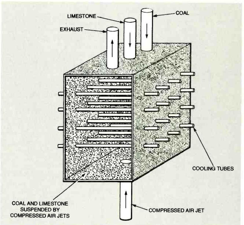
FIG. 9—CONSTRUCTION OF A FLUIDIZED BED COAL FURNACE. Thermocouples are positioned to monitor and control temperatures in the system.
