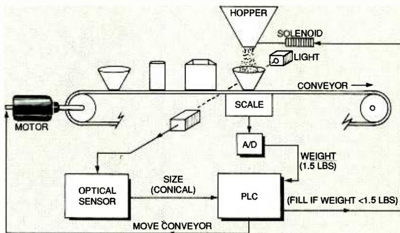
FIG. 13—VARIETY OF CONTAINERS are automatically filled. PLC is connected to an optical sensor and an A/D converter to be able to do this automated task.
