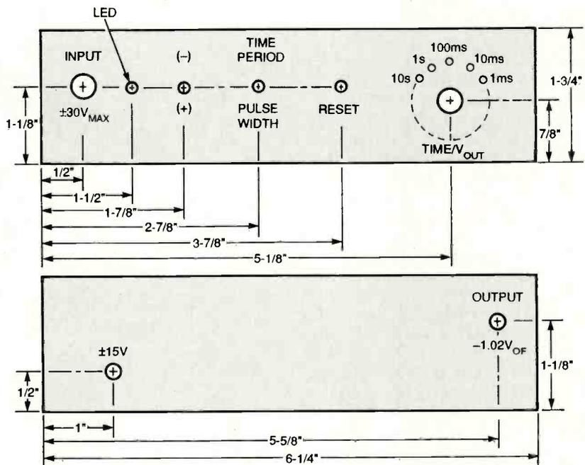
FIG. 3—HOLE DRILLING AND LABEL location diagram for the specified project case.
