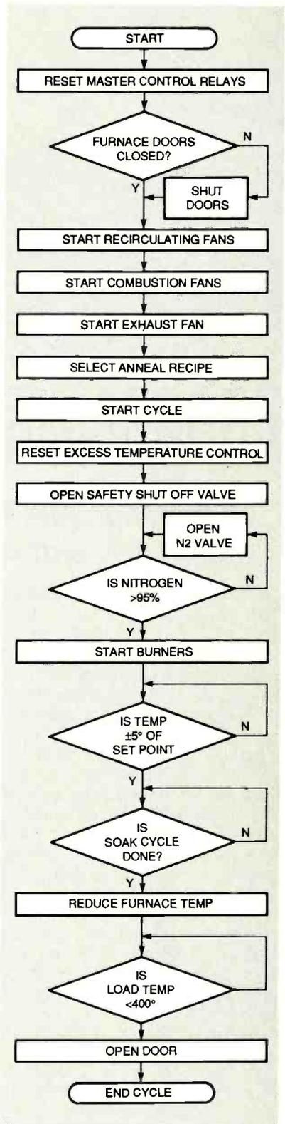
FIG. 2—FLOW CHART for a typical annealing furnace.
