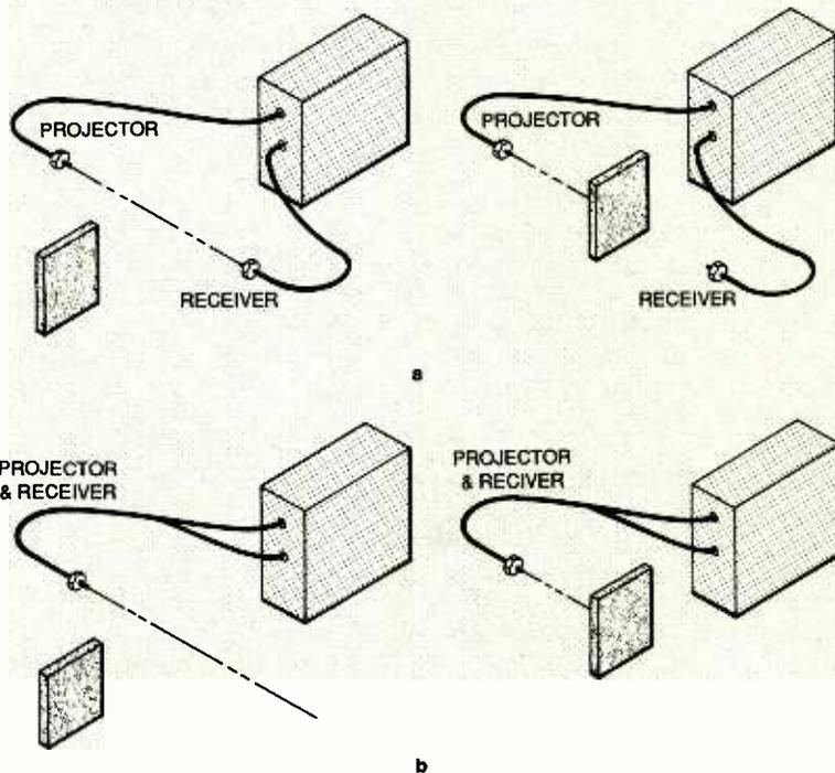
FIG. 14—TWO KINDS OF OPTICAL SENSORS. Through-beam sensor uses separate projector and receiver (a). Diffuse-reflected light sensor combines projector and receiver into one unit (b).
