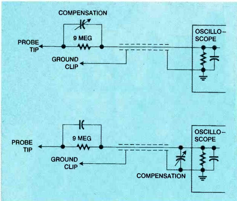
Fig. 1—TWO TYPES OF 10:1 low-capacitance oscilloscope probes.
