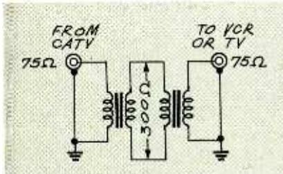
FIG. 3—USE TWO LINE-MATCHING video transformers to isolate CATV ground from home video components.
