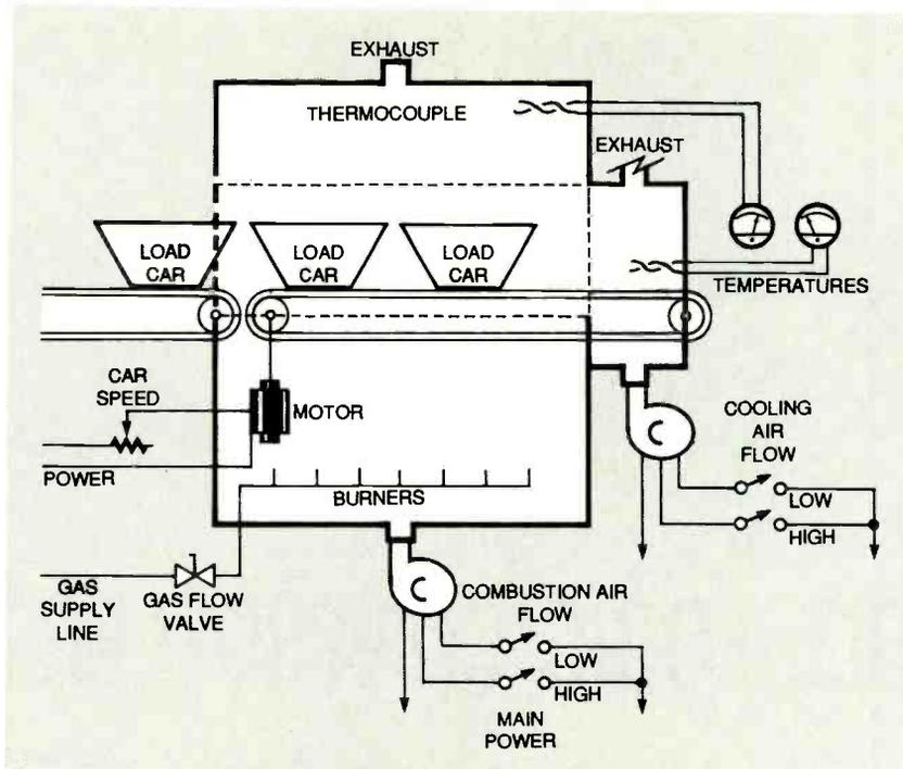
FIG. 1—SIMPLIFIED DIAGRAM OF A MANUAL FURNACE shows all the adjustments and measurements that must be controlled to insure proper operation.
