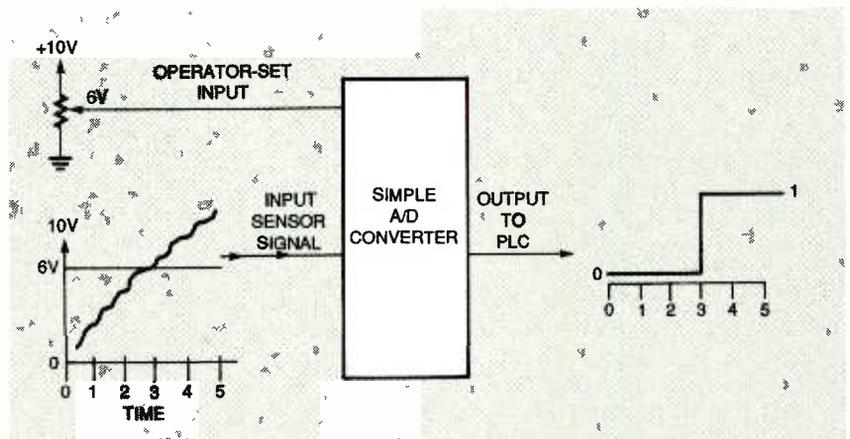
FIG. 12—BASIC EXAMPLE OF A/D CONVERSION as it might be used in an industrial application.
