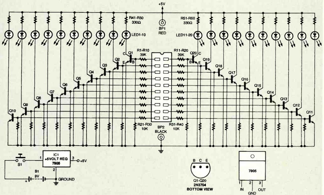
FIG. 1—SCHEMATIC DIAGRAM for the Analogic IC Tester reveals possible mirror-image layout on printed-circuit board.
