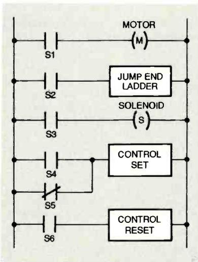
FIG. 7—THESE LOGIC-LADDER ELEMENTS include programmable control functions.
