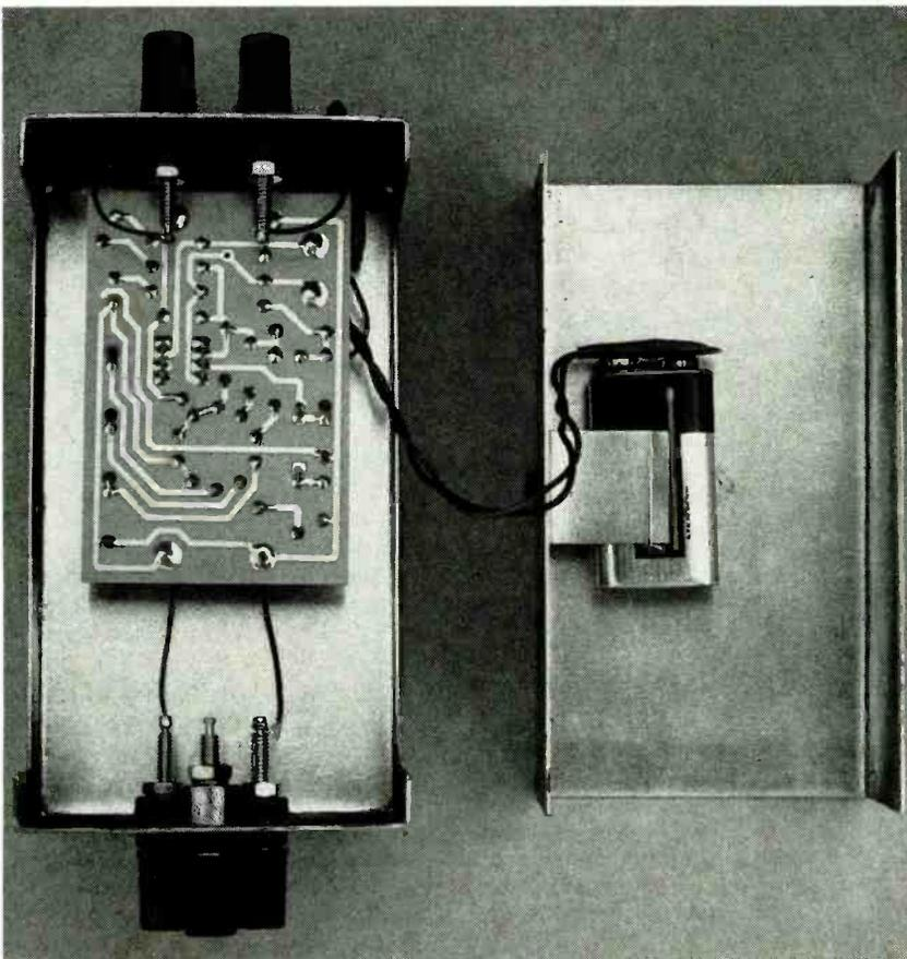
70 FIG. 5—ASSEMBLED CIRCUIT BOARD is mounted in its case.
