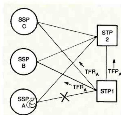
**FIG. 6—NETWORK MANAGEMENT** automatically re-routes messages in the event of failures.
