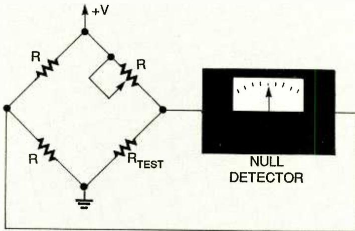
FIG. 1—A NULL DETECTOR can be used to verify that a bridge is in balance.
